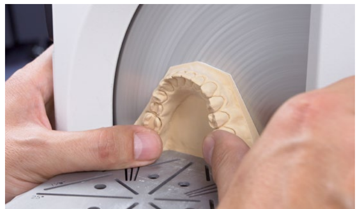
Powerful wet and dry trimming with minimum vibrations
