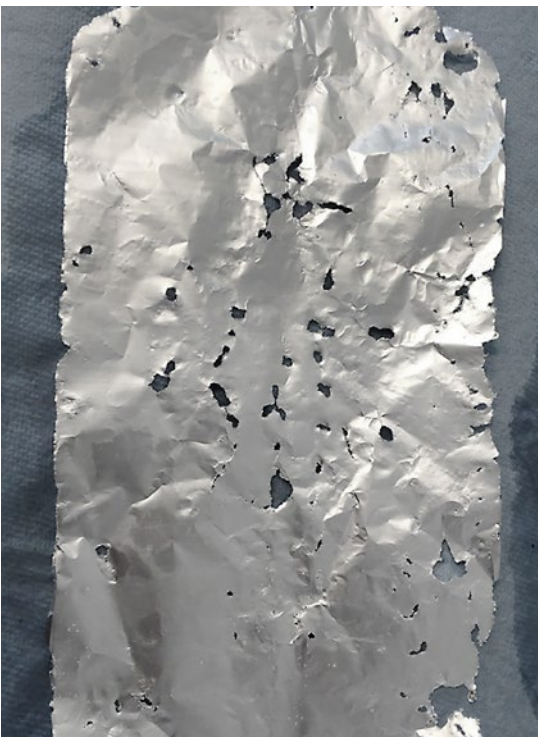
Example of a piece of aluminum foil after the ultrasound test in the Easyclean
